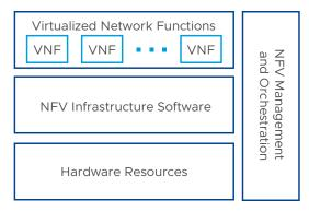
FIGURE 3: VNFs running in an NFV architecture.
