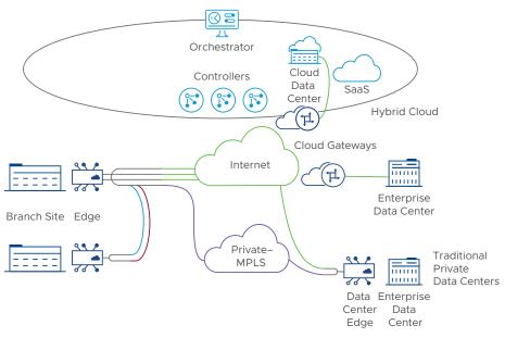
FIGURE 4: Architecture of a VMware SD-WAN solution.
