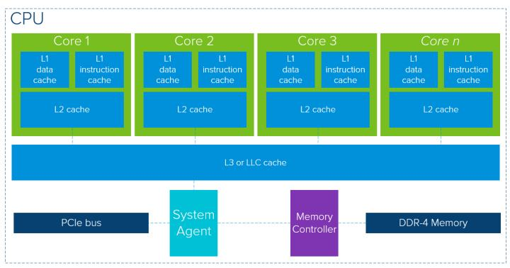
A single CPU package consists of cores that contains separate data and instruction layer-1 caches, supported by the layer-2 cache. The layer-3 cache, or last level cache, is shared across multiple cores. If data is not residing in the cache layers, it will fetch the data from the global DDR-4 memory. The numbers of cores per CPU can go up to 28 or 32 that run up to 2.5 GHz or 3.8 GHz with Turbo mode, depending on make and model. Caches sizes range up to 2MB L2 cache per core.
