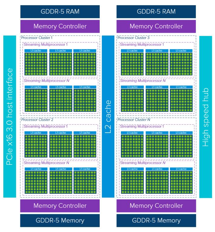
A single GPU device consists of multiple Processor Clusters (PC) that contain multiple Streaming Multiprocessors (SM). Each SM accommodates a layer-1 instruction cache layer with its associated cores. Typically, one SM uses a dedicated layer-1 cache and a shared layer-2 cache before pulling data from global GDDR-5 (or GDDR-6 in newer GPU models) memory. Its architecture is tolerant of memory latency.
