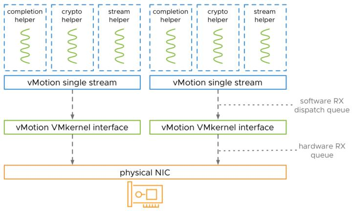
A single vMotion stream has an average bandwidth utilization capability of 15 GbE. When we look at various NIC speeds, that lead to the following:
