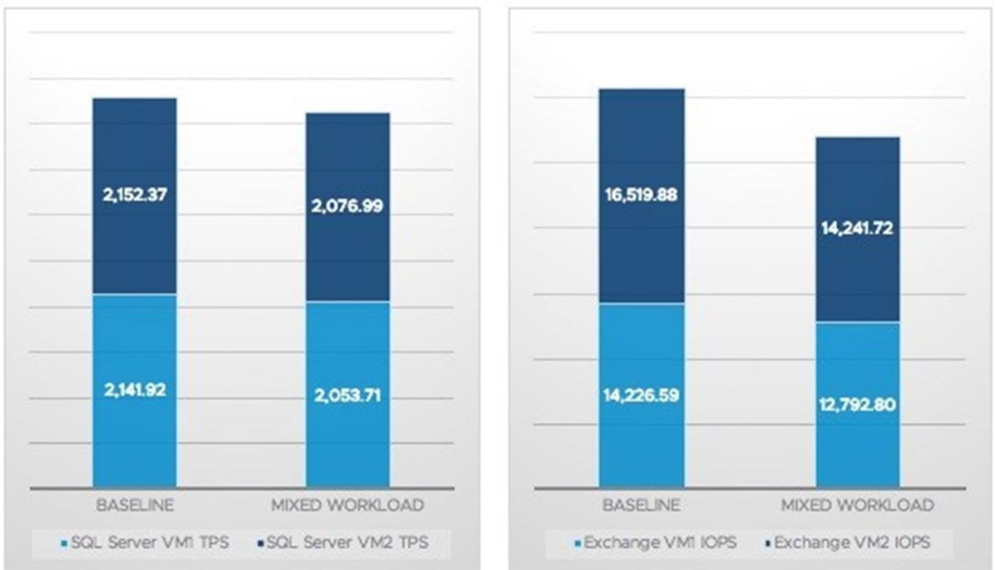
Figure 4. Mixed Workload Test Result of SQL Server and Exchange Standalone Performance
