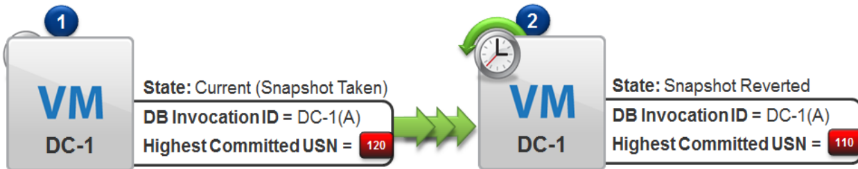
Figure 3. Domain Controller Reverted to Previous Snapshot
