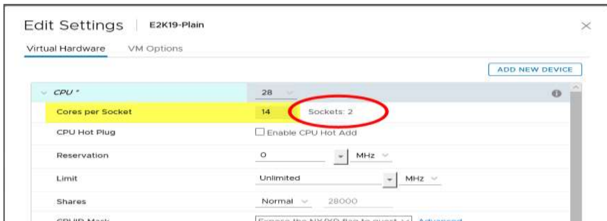
Figure 2. New Virtual Machine CPU Allocation Recommendation
