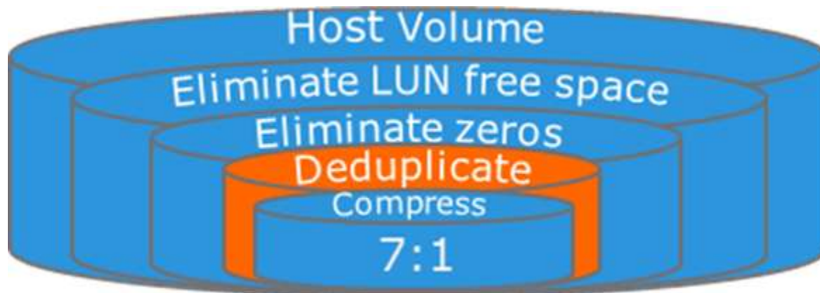
Figure 10 - Data Reduction Ratio on XtremIO
