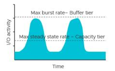
The performance maximums of your vSAN hosts will be somewhere in between the maximum burst rate, and the maximum steady-state rate. Synthetic testing for long periods using HCIBench will stress the environment enough to show these approximate values when looking at the time-based graphs. Production workloads may hit these maximums in an undersized design.
