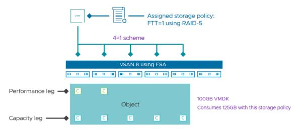
For clusters with fewer than 6 hosts, it will use a scheme of 2+1, spreading the data and parity fragments across at least 3 hosts. While this consumes a bit more capacity to make the data resilient (1.5x the capacity of the primary data), it is MUCH more space efficient than mirroring (2x capacity of the primary data), and can run on clusters with as few as three hosts, while also not impacting performance in any way. This makes RAID-5 an ideal choice for smaller clusters powered by the ESA.
