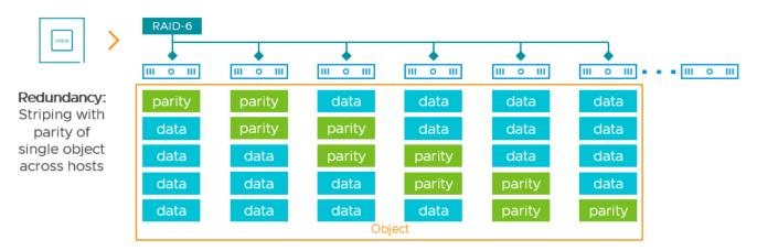
A 4+2 scheme allows vSAN to suffer the failure of two hosts for the hosts that are used to store this given object while maintaining availability of the object. The most significant difference with the ESA and RAID-6 is the complete elimination of CPU and I/O amplification that occurred with RAID-6 in the OSA. *In the ESA, RAID-6 is your best option for offering supreme levels of storage resilience while maintaining very good space efficiency, and no compromises on performance.*
