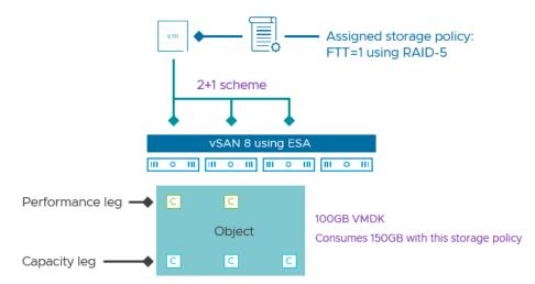
As a result of effective behavior of erasure codes in the ESA, RAID-5/6 erasure coding should be the data placement schemes of choice when the topology supports it. For stretched clusters, and 2-node topologies will still require the use of RAID-1 mirroring to protect the data across a site, or host respectively, but the secondary levels of resilience for these topologies can use erasure coding.
