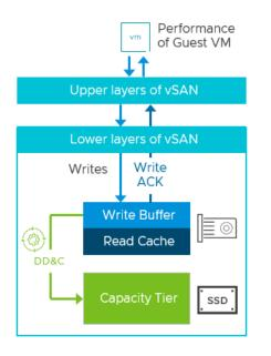
Implementing DD&C in this manner prevents the performance penalties found with inline systems that perform the deduplication prior to sending the write acknowledgment back to the guest. It also avoids the challenges of deduplicating data already at rest. While the DD&C process occurs after the write acknowledgment is sent to the guest VM, enabling it in vSAN can impact performance under certain circumstances, which will be discussed below.
