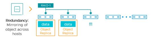
Data mirroring is a simple data placement scheme that uses minimal computational overhead but comes with the tradeoff of using an equal amount of capacity somewhere else in the cluster to protect the object at the level of resilience you desire.
