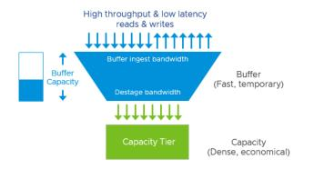
A two-tier system like vSAN has two theoretical performance maximums. A burst rate, representing the capabilities of buffer tier, and the steady-state rate, representing the capabilities of the capacity tier. The underlying hardware at each tier has a tremendous influence on the performance capabilities of each tier, but software settings, applications, and workloads can impact performance as well.
