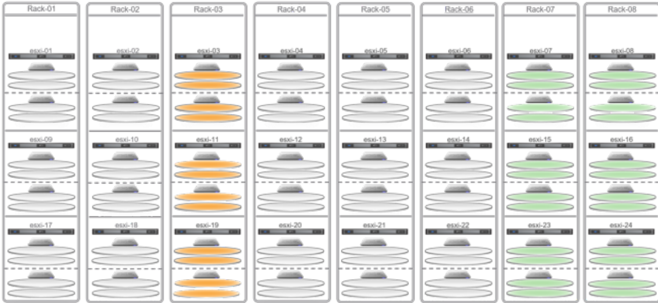
24 Host vSAN - 8 Racks, 3 hosts per rack, 2 SSD's, 4 HDD's per host & VM policy of #FTT=2, FTM=RAID6 Failure Domain 1 = Rack-01 (esxi-01, esxi-09, esxi-17), Failure Domain 2 = Rack-02, etc.
