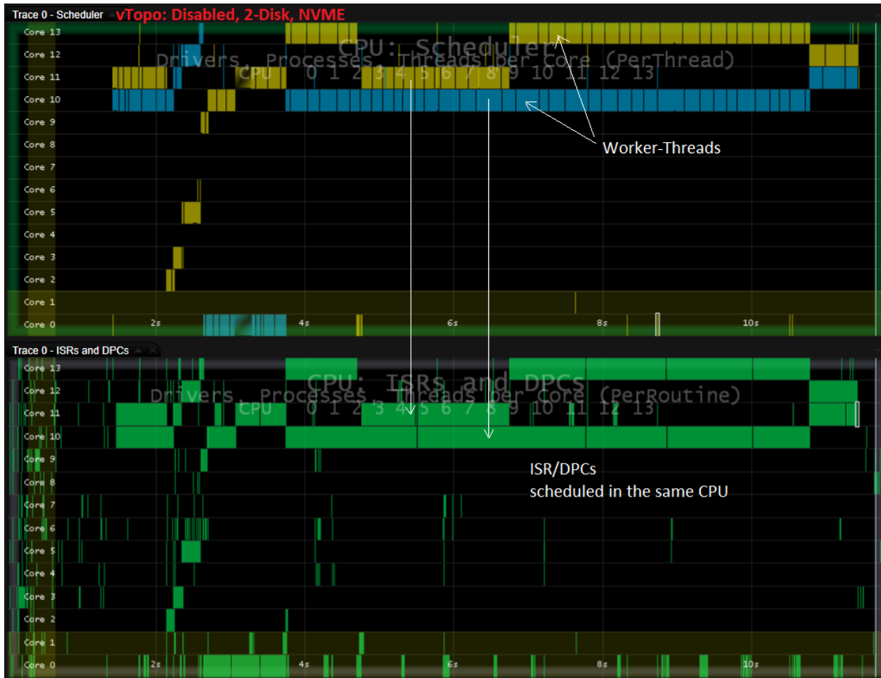
Figure 7. CPU scheduler and ISRs and DPCs view in Media eXperience Analyzer without virtual topology
